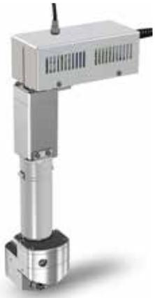
The robust and powerful Zünd Power Rotary Tool (PRT) was developed specifically for cutting challenging materials economically and reliably. The materials suitable for cutting with the PRT range from fiberglass to aramid. The tool can be set to 3 rpm levels -100 %, 75 %, and 50 % of the maximum. This allows for cleanly cutting very tough materials as well as those with low melting points.
